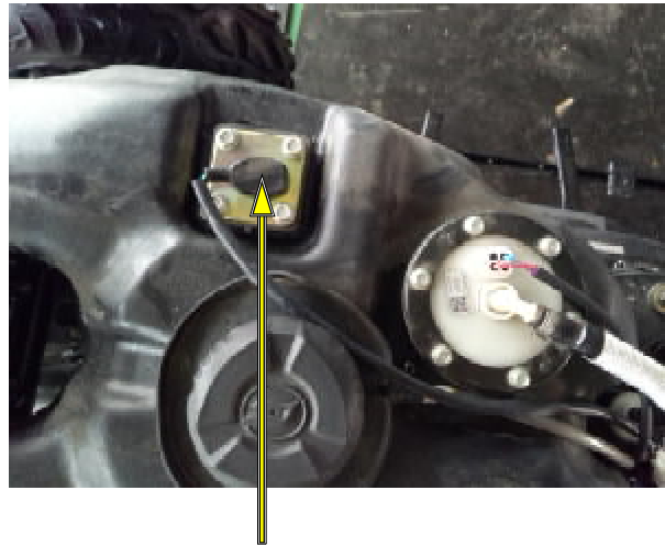
Fuel Sensor connector
