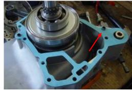
Install the cam chain, cam chain adjuster slipper and secure it with the bolt.
