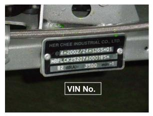
The VIN (Vehicle Identification Number) is attached to the lower front right side of frame behind the frame number.
