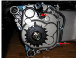
Remove gear shaft arm.
