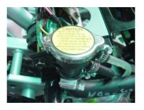
Check the level of coolant in the reserve tank and fill to the correct level if the level is low.
