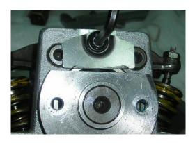
Push the cam chain adjuster push rod back into the adjuster body by pressing the tab down.
