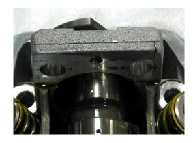
Install intake and exhaust rocker arm to cylinder head.
