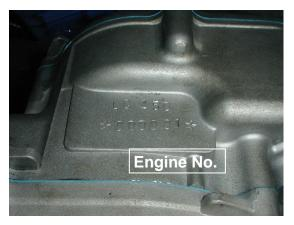
The engine serial number is stamped on the upper rear right crankcase.
