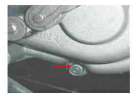
Remove drive sprocket.
