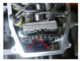
Remove the four cylinder head cap nuts and four copper washer.
