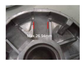
Check the driver face for wear or damage.
