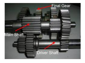
Inspect gear shaft arm for abnormal wear or broken teeth.
