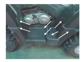
Raise up the fender and pull to back to remove the rear fender.
