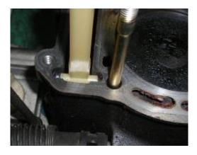
Remove the cam chain adjuster base and gasket from the cylinder.
