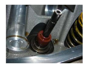
The springs' tightly wound coils should face in toward the combustion chamber.
