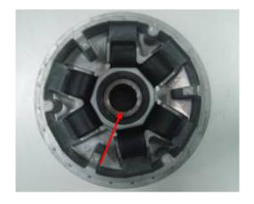
Apply grease to the drive pulley collar.
