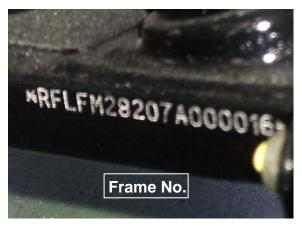
The frame serial number is stamped on the lower front right side of frame.
