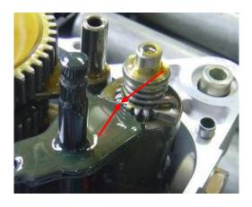
Install the dowel pins and a new gasket, add specified gear oil to gear box.
