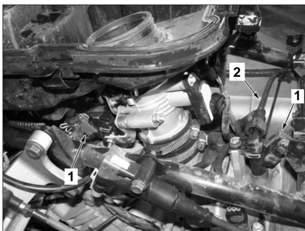
1. Injector Connector 2. Fuel Line
