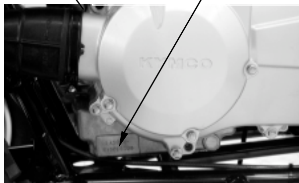
Location of Engine Serial Number
