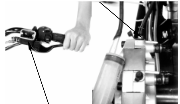
Reservoir (Front Left Lever)Bleed Valve (Pedal)
