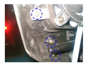
Remove head lamp couplers  $\,\,^{,}$  and then remove front bumper
