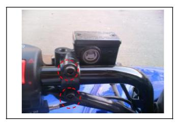
Install the brake lever, and connect leads to brake light switch.
