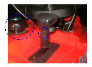
Remove 4 screws  $\,^{,}$  and then remove fuel tank cover
