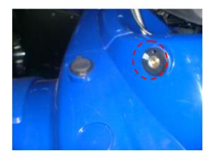
Remove power source couplers  $\,\,^{,}$  and then remove front body cover
