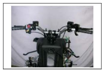
Loosen the socket bolts for the front brake master cylinder, and remove front brake master cylinder.
