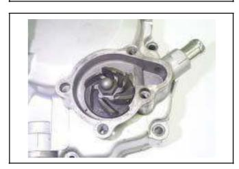
Install the dowel pin and new gasket. Install the water pump cover with 4 bolts.
