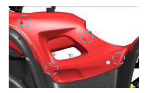
Remove screws from right or left foot board (each side 8 screws)
