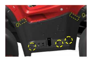
Remove bolts from right or left front internal fender (each side 5 bolts), and then remove right or left front internal fender
