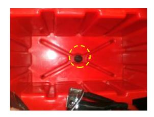
Remove 1 nut from bear reflector assembly (each side 1 bolts)
