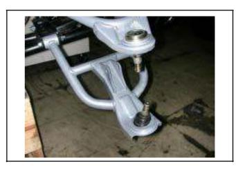
Loosen upper suspension arm nuts, remove swing arm bolts.
