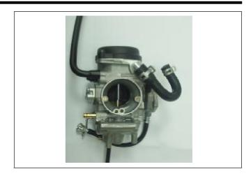
Remove air cut-off valve cover 2 screws, spring and valve.
