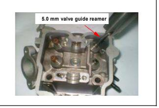
Measure and record each valve guide inner diameters.
