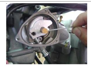
Disconnect the starter cable. Remove the carburetor.
