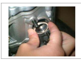
Apply sealant to the muffler mounting bolt Install muffler. Pay attention don't damage the connector.
