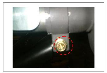
Apply sealant to the muffler mounting bolt to the muffler fixed bolts and tighten them.
