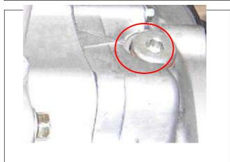
Turn the crankshaft and let the "T.D.C line" on the rotor with index mark.
