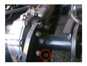
Place an oil pan below the case of final gear set. Remove the drain blot. Remove the filler cap Drain oil nut.
