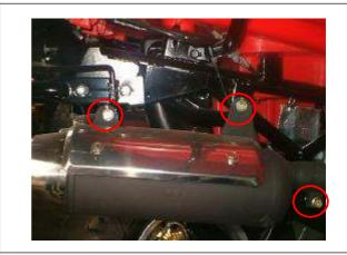
Remove the exhaust pipe.
