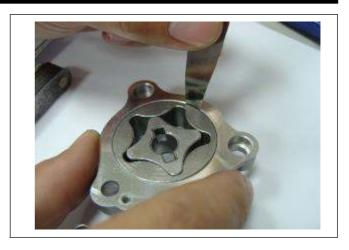
Check clearance between inner and outer rotors.
