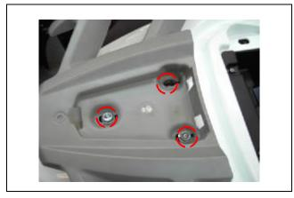
Remove the bolts from rear body cover. (each side)
