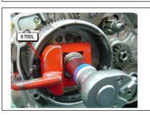
I Install the output drive gear by installing the snap ring.
