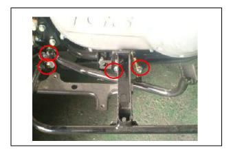
Remove 3 bolts form rear frame And 2 bolts from muffler.
