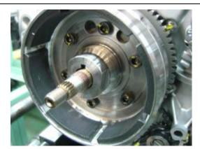
I Tighten the generator rotor nut to the specified torque with the special tool.
