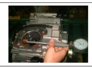
Measure the inner diameter of piston pin hole. Service Limit: 20.02 mm Calculate clearance between piston pin and its
