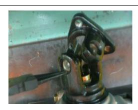
After reassembling the universal joint assy. Check the joint assy. Movement smoothly. If movement have a large resistance. Tapping the bearing with the plastic mallet lightly.
