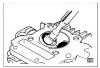
**Cylinder Head Reassembly** Lubricate valve stem with engine oil, and then insert the valve into valve guide.
