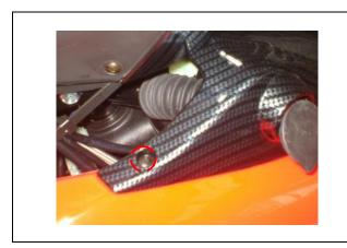
Remove 8 screws from right or left side cover. (each side 4 screws)
