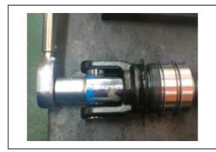
Stake the nut with a punch. After The tooth contact and backlash have been adjusted and checked.
