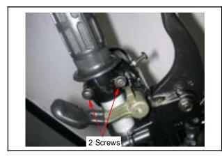
Loosen the socket bolts for the front brake master cylinder, and remove front brake master cylinder.
