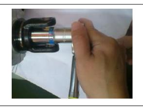
Remove the bearing by tapping with the hammer and tool.
