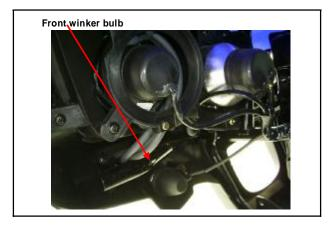
Replace with new front winker light bulb. (12V 21W)
