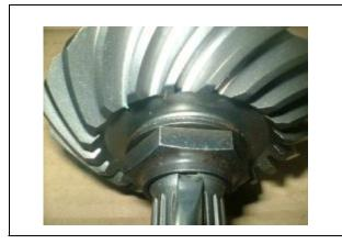
Using a vise held the driven output front shaft and remove the nut.
