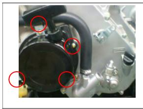
Remove the valve timing check plug.
