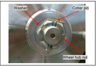
Remove cotter pin, wheel hub nut and washer. Remove wheel hub and brake disk.
