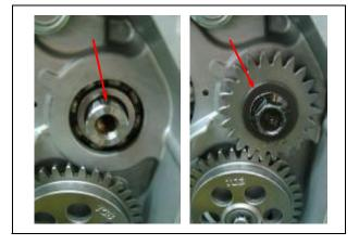
I Tighten the oil pump drive gear bolt to the specified torque.
