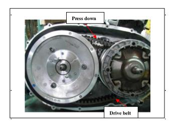
Install Movable drive face, and nut. Loosen the 2 screw.
