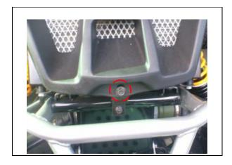
Remove bolts from first housing. (each side 1 bolt)
