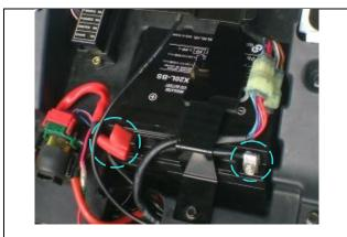
Remove 2 bolts from battery fixed. Then, remove cable.
