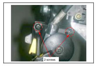
Remove switch wire band. Remove handle mounting bolt, and then remove the handle upper holder, handle.
