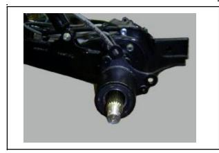
Remove tow ball mount 4 bolts (2 bolts each side)
