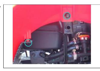
Remove screws (each side) from the part of front body cover, and then remove front body cover.
