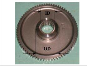
Check the starting reduction gear and shaft for wear or damage.
