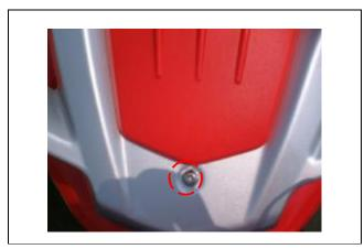
Remove 3 bolts from tail carrier, then remove tail carrier.
