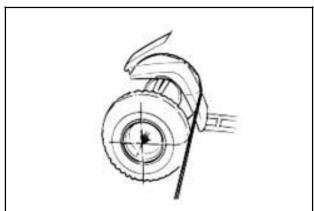
If the toe-in is out of standard, adjust it by hanging the length of the tie-rods equally by turning the tie-rod while holding the ball joint.
