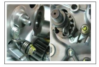
I Install the gearshift shaft by aligning the punched mark with the center of the cam driven gear.
