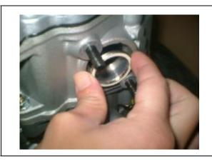
Apply sealant to the muffler mounting bolt Install muffler. Pay attention don't damage the connector.
