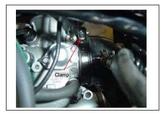
Loosen the clamp strip of air cleaner, and then remove the air cleaner vapor hose.
