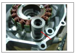
Using an shaped tool to check the oil pressure valve Operation. If the piston does not operate, replace the new one.
