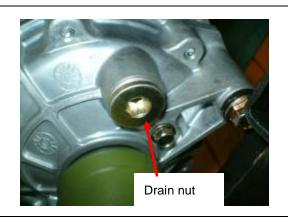
Remove drain bolt, filler nut and drain oil out. Tighten the drain bolt to specified torque. Pour the oil through the filler hole. Tighten the filler cap to the specified torque,
