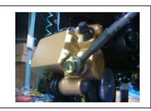
Remove two caliper bolts and the caliper.
