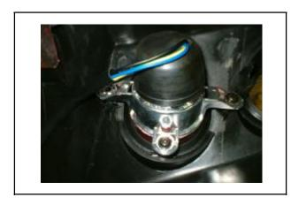
Replace with new taillight bulb. (12V 5W/21W)
