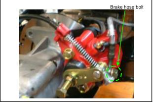
Remove two caliper bolts and the caliper.
