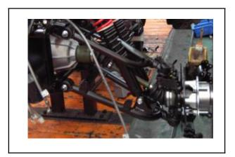
Loosen upper suspension arm nuts, remove swing arm bolts.
