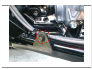
Remove bolts from rear protector (each side 1 bolts), and then remove rear protector
