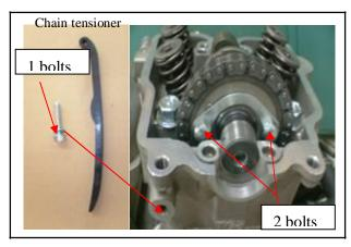
Remove cam shafts.
