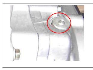
Turn the crankshaft and let the "T.D.C line" on the rotor with index mark.
