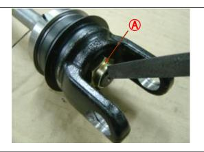
I Stake the collar of the nut (A) into the notch in the shaft.
