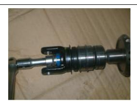
Stake the nut with a punch. After The tooth contact and backlash have been adjusted and checked.
