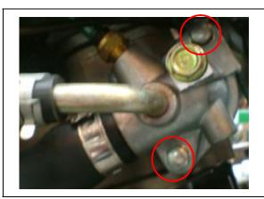
Remove the spring bolt and remove the cam chain pensioner adjuster assy.
