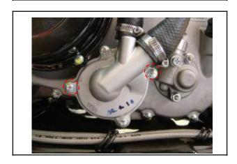
Remove coolant filler pipe.
