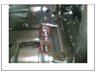
Remove 2 bolts from front protector, and then remove front protector.
