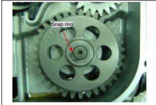
Make sure that pump shaft can be rotated freely. Remove 3 screws on the oil pump, and then remove oil pump.
