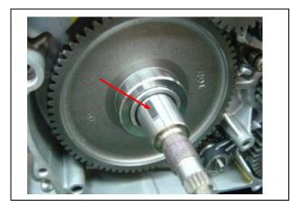
I Install the one way clutch and generator rotor sets.
