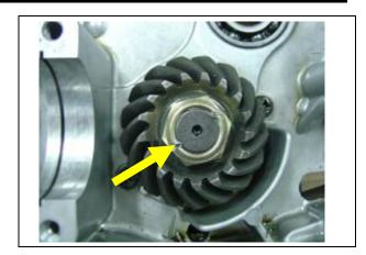
Rear output shaft nut:100 N  $\cdot$  M(10.0 kgf- m, 73 lb-ft) Drive bevel gear nut:100 N  $\cdot$  M(10.0 kgf- m, 73 lb-ft)
