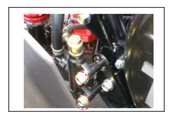
Install brake push rod to the brake pedal, and install pin and clip.
