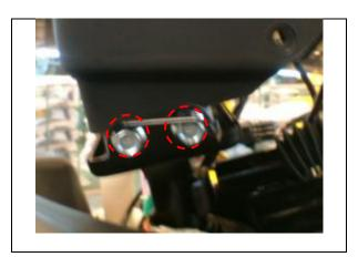
Remove speedometer assembly couplers, and then remove upper bracket assembly.
