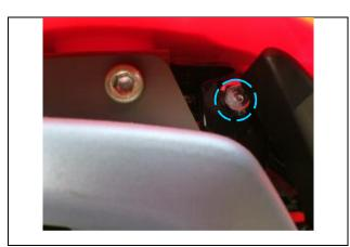
Remove 4 screws (each side 2 screws) from number-plate bracket.
