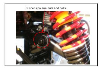
Loosen under suspension arm nuts, remove swing arm bolts.
