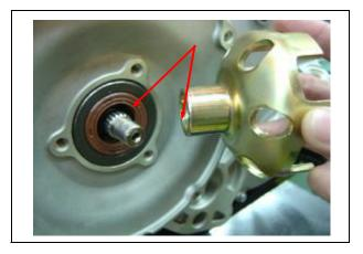
I Tighten the starter cup nut by using a suitable bar.
