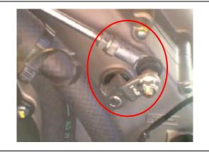
Remove the connector of lead wire. Remove the signal generator lead wire connector and generator lead wire connector.
