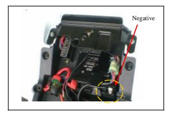
Remove starter motor cable. Loosen the lock bolts and remove the starter motor.
