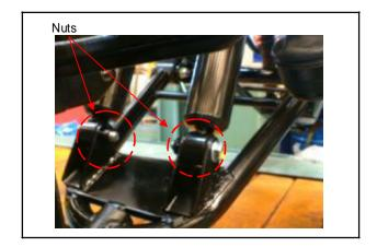
Remove front cushion upper bolt nuts, and remove the bolts and cushions.
