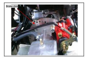
Remove the brake disk from rear wheel axle. Check the disk for deformation and bend.
