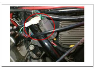
Remove the spark plug cap.
