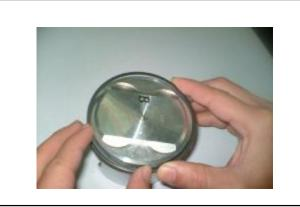
Place piston rings respective into cylinder below 20 mm of cylinder top. In order to keep the piston rings in horizontal level in cylinder, push the rings with piston.
