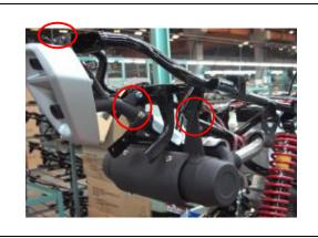
Loosen the bolt and take down the muffler.
