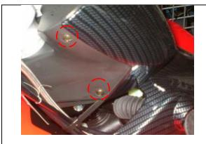
Remove bolts from upper bracket assembly. (each side 2 bolts)
