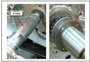
I Install the water pump gears and tighe the nut
