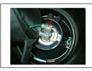
Take out the bulb connector and the bulb. Replace with new bulb if necessary. (Main beam H3 12V 55W)
