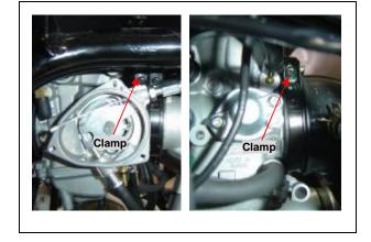
Loosen the carburetor side cap 3 screws. Remove cap.
