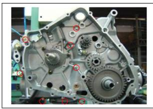
I Check the each shaft rotates smoothly after the crankcase bolts have been tightend.
