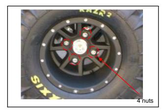
Remove the front wheel nuts, and then remove front wheels.
