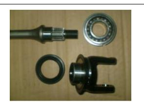
Rear universal joint disassembly. Remove the c-rings from the universal joint assy.
