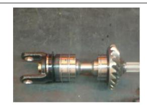
Unlock the nut with a chisel.
