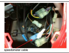
Remove 4 nuts and meter wire, and then remove speedometer and fuel meter.
