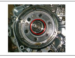
Install reduction gear shaft and reduction gear.
