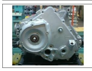
Note: Align the water pump shaft indent with the water pump gear shaft.
