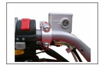
Install the brake lever, and connect leads to brake light switch.
