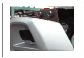
Install 2 bolts(each side 1 bolts) from rear frame.
