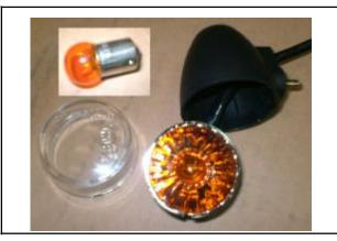
**Replacing Bulb of Position Light**Pull out the position light bulb seat.
