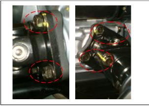
Remove the engine mounting bolts and nuts. Remove the engine mounting bracket.
