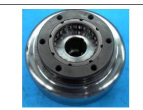
Install starting clutch driven gear onto one way clutch. Hold flywheel and rotate starting clutch gear. The starting clutch gear should be rotated in C.C.W direction freely, but not C.W direction. (View as shown in this figure.)
