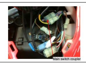
Remove speedometer cable, and then remove meter set, main switch and handle cover
