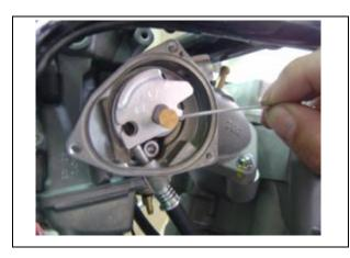
Disconnect the starter cable. Remove the carburetor.
