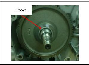
Hold the flywheel by drive face with universal holder, and tighten flywheel nut.
