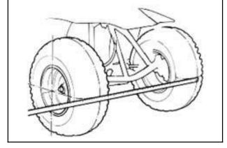
Carefully to move the vehicle back, let the wheels turn 180 degree, so the marks on the tires are aligned with the axle center height.
