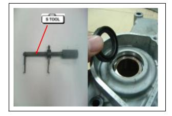
I Install the oil seal with the special tool.
