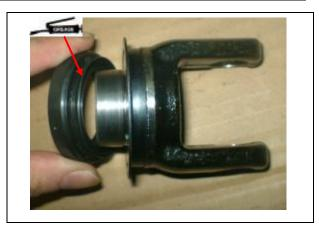
Insert the bearing to the joint and turning the joint. If excessive play is noted, must be replace the new bearing.
