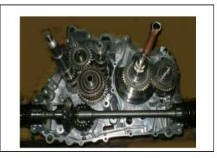
Remove the c-ring from the universal joint assy. Remove the driven output front shaft with a chisel.
