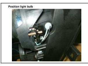
Replace with new position light bulb. (12V 5W)
