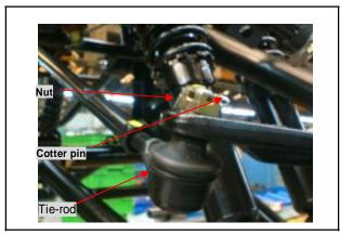
Remove cotter pin and ball joint nut. Remove upper and under ball joints by ball joint driver.
