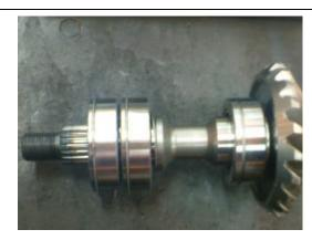
Apply grease to the bearing and seal lip.
