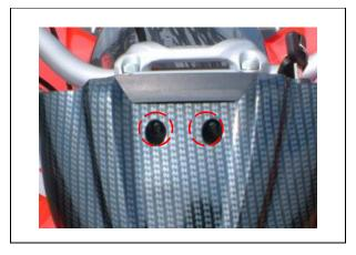
Remove 4 bolts from handle bar front cover. (each side 2 bolts)
