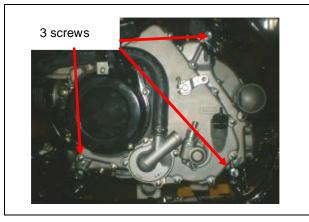
Remove the flange bolts and take down engine bolster. Remove the engine from the right side.
