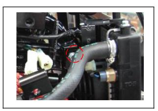
Remove coolant outlet pipe.
