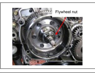
Remove starter reduction gear and shaft. Pull out flywheel with A.C.G. flywheel puller.
