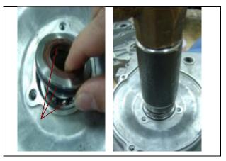
I Apply a small quantity of Loctite 262™ (Thread locker) to the screws and install the bearing retainer.
