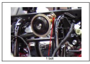
Apply 12 V power source to two terminals of the horn, the horn should sound. Replace the horn if necessary.
