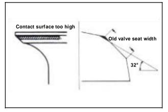
If the contact surface too high, grind the valve seat with 32° cutter.
