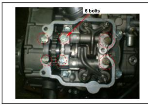
Remove cam sprocket bolts and then remove the sprocket by prying chain out.
