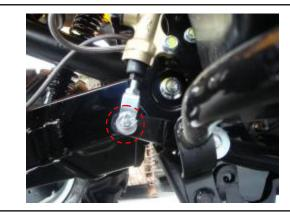
Install fluid hose and clamp. Connect brake hoses with 2 new washers. Tighten the brake hose bolt to the specified torque value.
