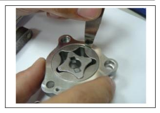
Check clearance between inner and outer rotors.
