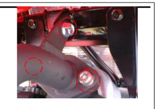
Install 2 bolts from muffler.
