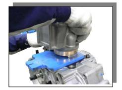
• Install Chain Guide 1 onto Cylinder.
