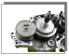
• Adjust the convex position on the end surface of Water Pump Shaft to meet with the groove on the end surface of Balancer Shaft (on Crankcase 1 side).
