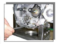
• Assemble Drum Shifter and related parts. Make sure the spring force and smooth operation by moving the ratchet pole with finger.
