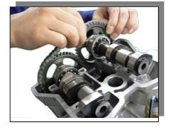
• Apply oil to Cam Support and install in position.
