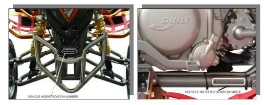
Whenever corresponding with DINLI about a particular issues, the engine number and serial number are important for vehicle identification.
