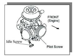
Readjust idle speed to specification.
